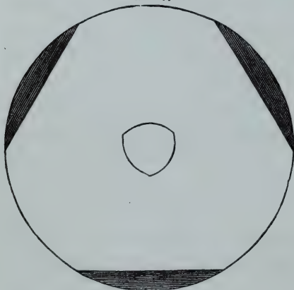
PLAN FOR CURING TRIANGULAR STAR-DISCS.
